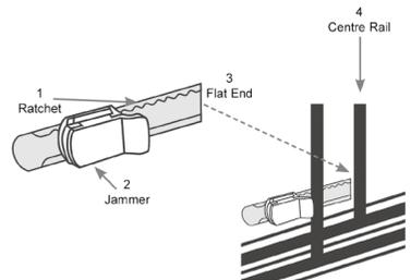
For the Jammer holder, repeat steps 2 and 3 as above. No pre-treatment is strictly needed as the holder shouldn't encounter any force, though you can wipe down the area if you wish.
