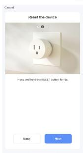
3. Press and hold the button for approx 5 secs until you hear a click, then release. The light should start flashing blue. Press Next.
